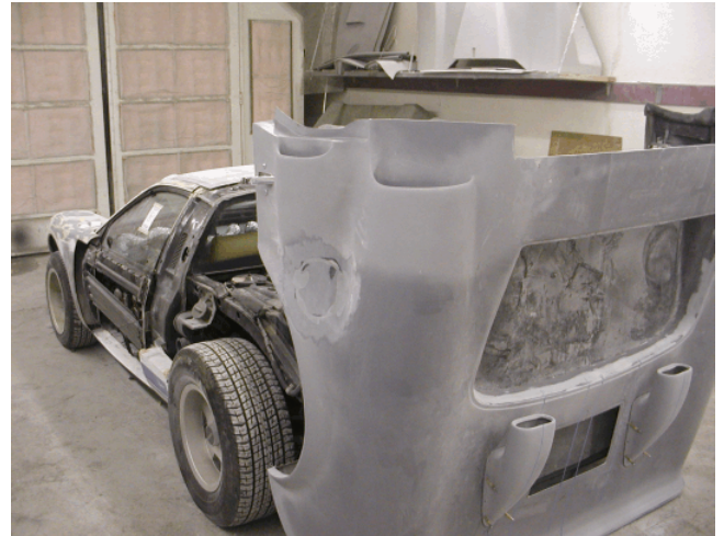
New rear body clip installed
